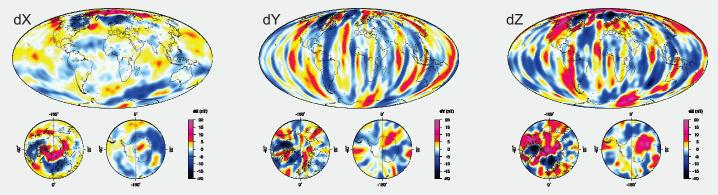
The above images show the differences between two independent models from Swarm A and Swarm B projected forward to January 1st, 2017 at the Earth surface for the magnetic Northward (X), Eastward (Y) and Downward (Z) components.
